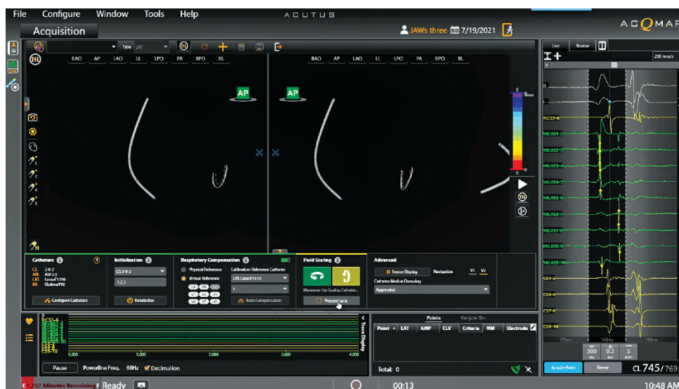
Figure 16-5. Move the catheter in the horizontal and vertical directions until the horizontal and vertical arrows turn green.
