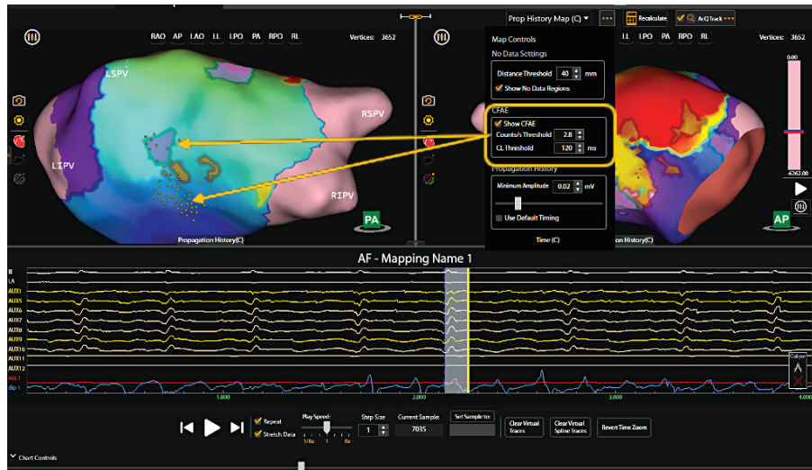
Figure 13-14 Check “Show CFAE” box to enable visualization of nodes with fractionated electrograms. These are shown as golden dots (yellow arrows) on the Propagation Map in the 3D Display based the CFAE algorithm settings (yellow box).
