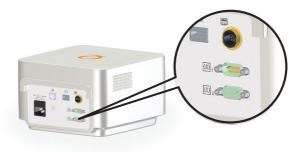
The Qubic RF is connected using the Qubic Force™ RS-232 Spy Cable.
